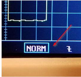
Short press repeatedly until the trigger type is highlighted, (second from the right at the bottom of the display), and use the adjustment knob to cycle between AUTO, NORMAl, and SINGle triggering mode.
