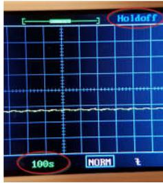
Trigger is disabled until portion of data buffer prior to display is filled with data. You may see this with long timebase values.
