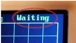
Trigger is waiting for scope signal to cross the threshold value in on the slope selected for triggering (rising or falling.)
