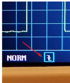
Short press repeatedly until the trigger edge is highlighted, (rightmost symbol at the bottom of the display), and use the adjustment knob switch between rising edge and falling edge triggering.
