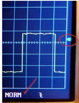
When NORMAl mode is displayed, press again to remove the highlight from the trigger mode, now turning the adjustment knob will change the trigger level. You will see blue arrow move up and down along the right edge of the display indicating the voltage threshold to trigger.
