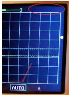
When AUTO triggering is selected in combination with a timebase greater than 50ms, triggering is disabled and the signal is scrolled across the display continuously.
